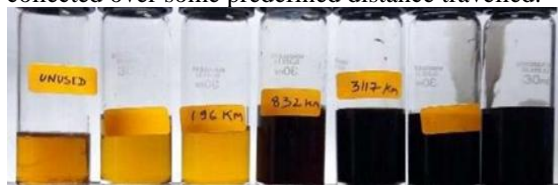
Fig 5: Various oil samples degraded over usage
