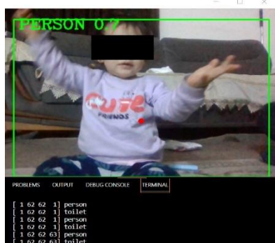
Figure 6b: Multiple Objects Detected, Only Person Marked by Bbox
