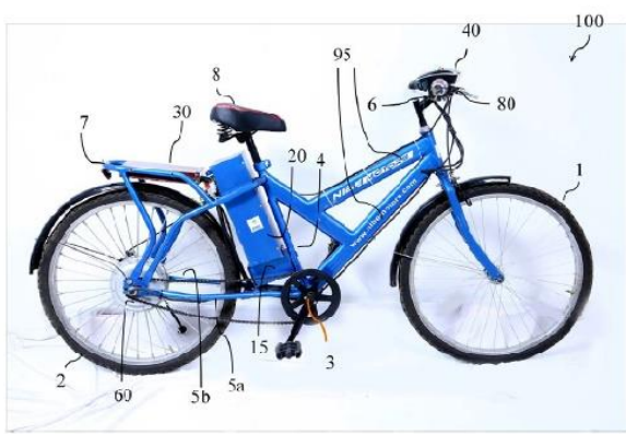
[Fig.1: (B) Picture of an Embodiment of the Electric Bicycle]
