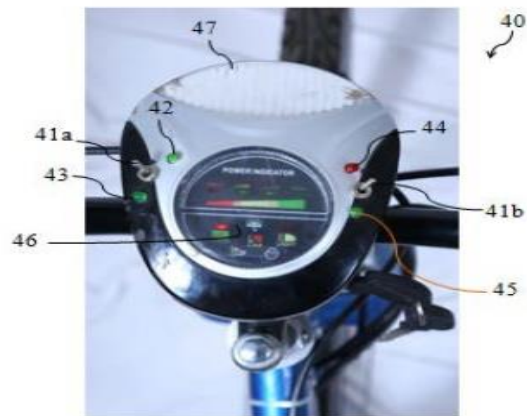
[Fig.4: (B) A Picture of an Embodiment of the Head Panel for Display and Controls]
