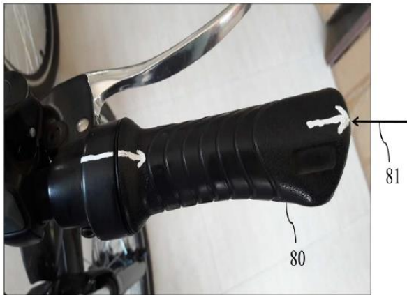
[Fig.3: (A) Pictures of an Embodiment of a Handle Housing the Hall Effect Speed Controlling Device of the Electric Bicycle]
