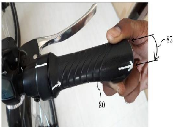
[Fig.3: (A) Pictures of an Embodiment of a Handle Housing the Hall Effect Speed Controlling Device of the Electric Bicycle]
