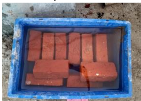
Fig. 9: Bricks Placed in Water for Water Absorption Test
