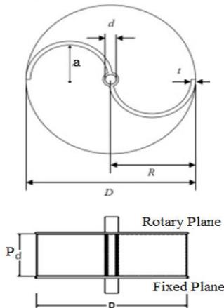
**Figure 2: The Schematic Diagram of the Modified Savonius Wind Turbine**
