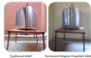
**Figure 10: PM-VAWT Model vs. Conventional VAWT Model**
