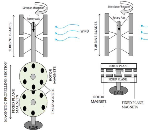
**Figure 6: Schematic Diagram of Permanent Magnet Propelled VAWT**
