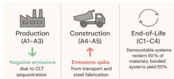
[Fig.3: Life Cycle Stages of Steel-CLT Systems. (Adapted from [6])]
