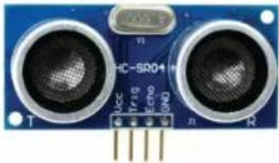
[Fig.1: Ultrasonic Sensor [19]]
