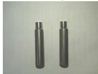
Figure 2 and figure 3 shows the Titanium Alloy Ti-6AL-4V before and after machining on Spark Erosion EDM.
