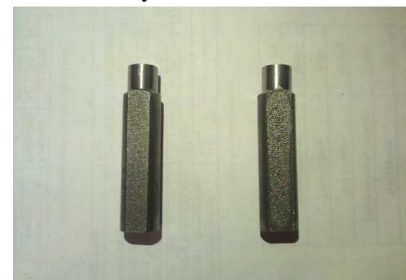
Figure 3: Titanium Alloy Ti-6AL-4V after EDM machining
