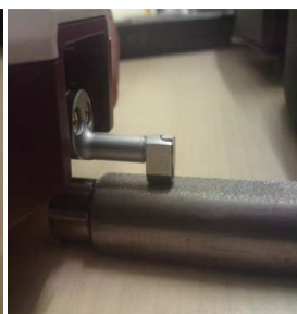
Figure 5 : Profilometer Measuring Surface roughness
