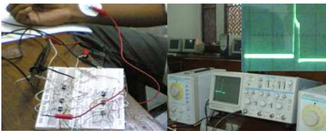
a. Testing amplified ECG      b. ECG waveform observed
