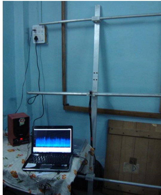
Figure 5: System setup showing the FM detector, Yagi-Uda antenna and laptop
