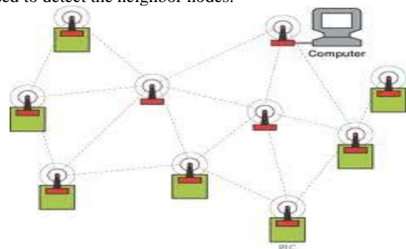
Figure 1: Multiradio WMN. A network often experiences wireless link failure and needs to reconfigure its settings.
