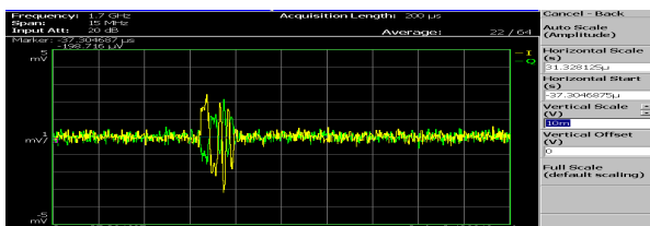
Figure 9: Received Pulsed barker waveform at the RTSA
