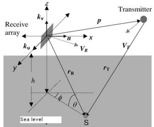
Fig.1: Bistatic radar geometry for sea clutter.
