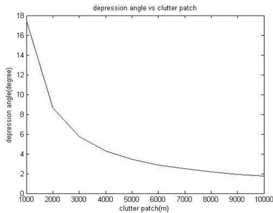
**Fig.5: Depression angle vs. clutter patch.**
