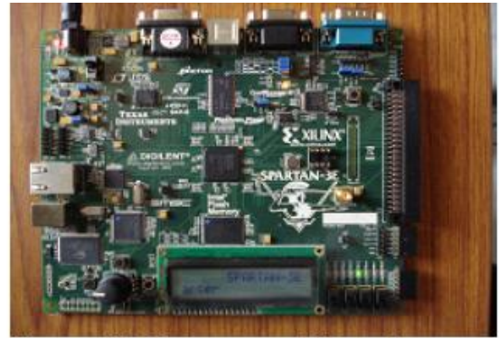
Fig. 8. FPGA Spartan 3 E Board
