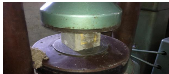
Figure: 5 Setup of Compression Strength Testing Machine
