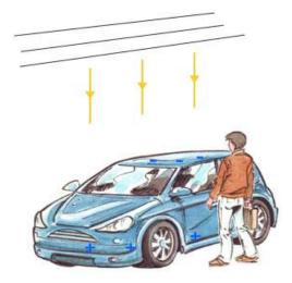
The car below the high voltage power line is subjected to an electric field: it does induce a displacement of charges. The car acquires a certain potential, different than that of the approaching person.
