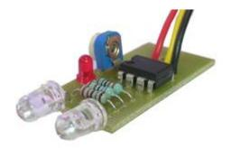
In the industry, there are conveyer belts either to transport the products or to convey the raw materials depending on the industry. This is modelled by the Conveyer belt in the prototype. Whenever a person picks up an item from the belt and IR Sensor based counter at the end of the belt counts the item.
