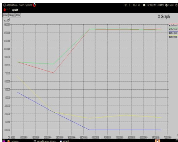
Figure 8 Comparisons of Total received packets in AODV and DSDV in sparse and dense medium
