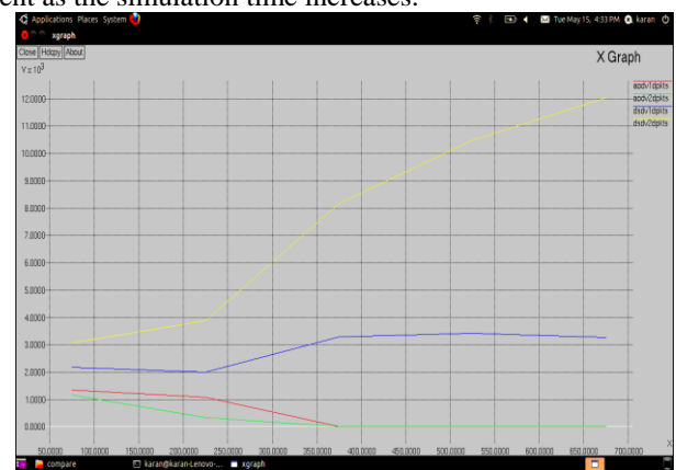
Figure 6 Comparisons of Total data packets in AODV and DSDV in sparse and dense medium
