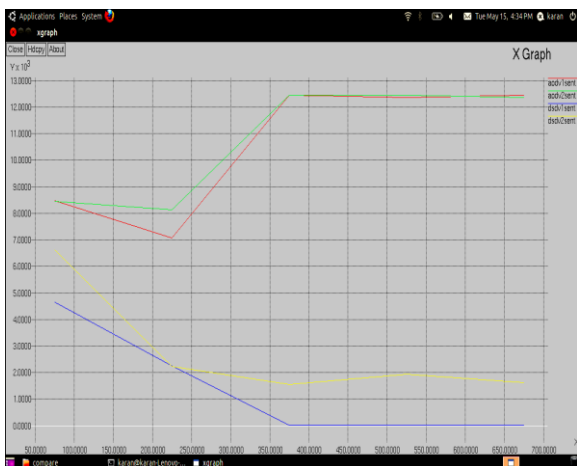
Figure 7 Comparisons of Total sent packets in AODV and DSDV in sparse and dense medium
