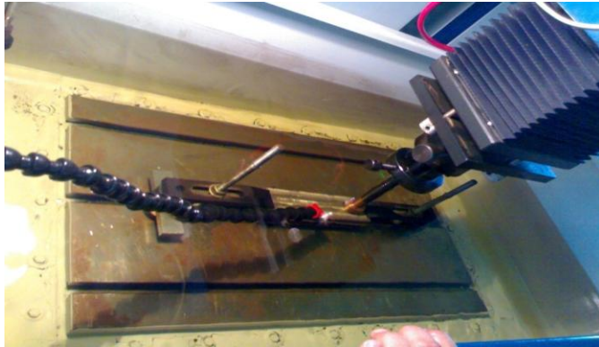
Fig IV. Setup of work piece & electrode
