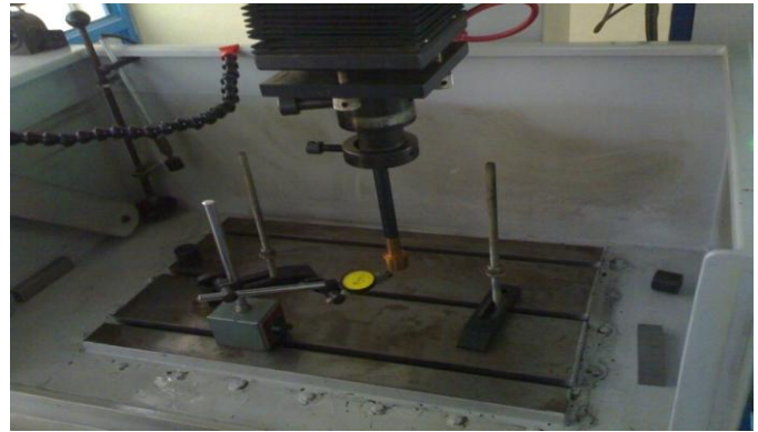
Fig III. To check level of the lower surface of the copper electrode
