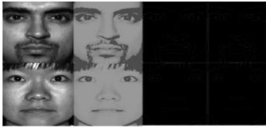
Fig. 4.1 Examples of the effect of different pre-processing methods. Column 1 shows the original image, 2 shows the output of gamma correction, 3 shows output of DoG filtering, 4 shows output of equalization of 2 subjects from Yale-B dataset.
