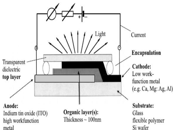
**Fig.1 A cross-section through the simplest form of an organic light-emitting diode(OLED). One of the two metallic or metallic-conducting electrodes must be semitransparent to permit the luminescence to exit the device. Typical thicknesses of the organic layer(s) between the electrodes are between 1nm and 100 nm.**
