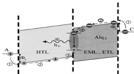
Fig.2 The structure and schematic energy diagram of a two-layer OLED. With a suitable choice of the layer thicknesses, recombination occurs in the emission layer (EML) Alq3 in the neighborhood of the HTL/Alq3 interface. Alq3 is simultaneously the electron transport layer (ETL). HTL is a hole transport layer. It can be made of e.g. NPB.
