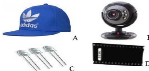
Figure 1: Elements of Head mounted Eye tracking system
