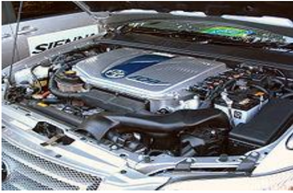
Toyota FCHV PEM FC fuel cell vehicle.
