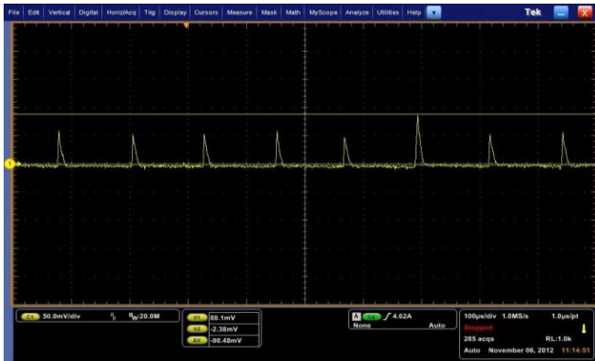
Fig.10: Output ripple at no load
