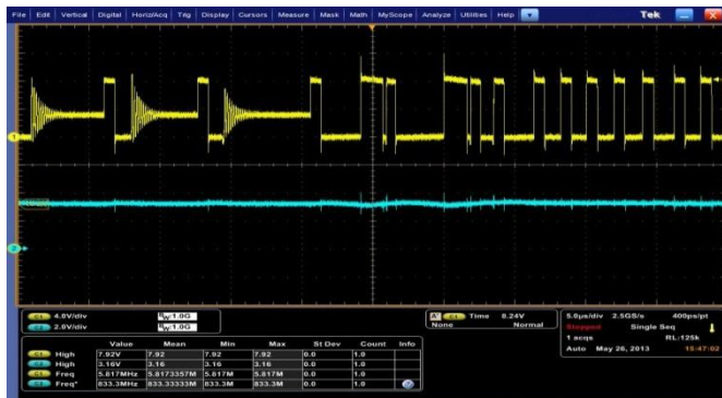
Fig.6: PFM to PWM transition of VR V4
