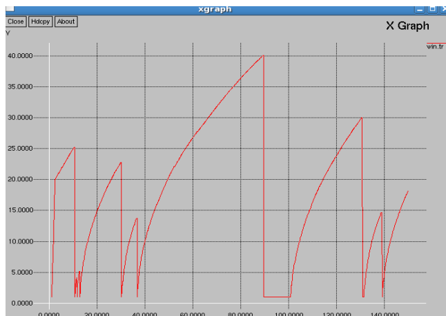
Fig. 6. Window size evolution for standard TCP with 9 nodes and maximum window size of 3
