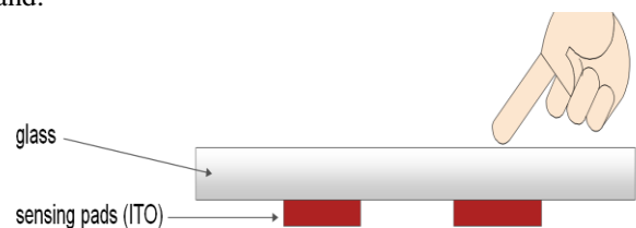
Figure 5 Capacitive touch screen with discrete sensing pads, consisting of one ITO layer [14]
