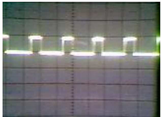
Fig.10. Pulse pattern for a speed of 1200 rpm
