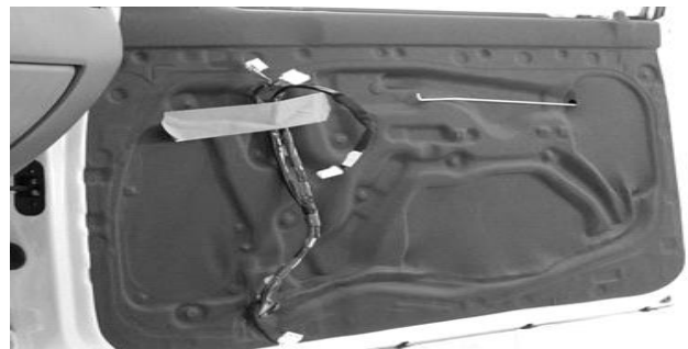
Fig.5.The completed door with VBD installed
