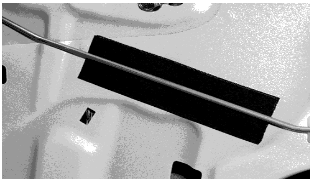
Fig.27.Gasket Foam installed behind a linkage rod to eliminate a potential rattle.
