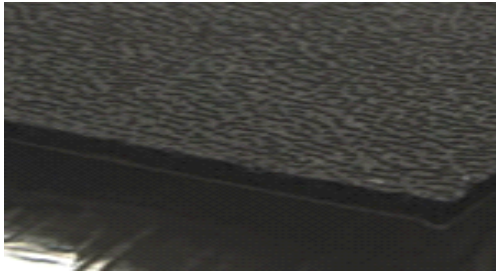
Fig.6. thick Vinyl Vibration Damping surface
