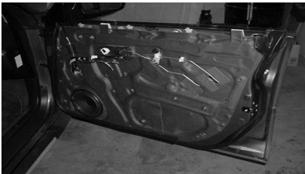
Fig.26.Passenger door treated with vinyl vibration damping material
