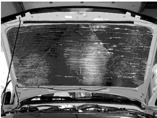
Fig.21. Thermo-Acoustic Liner applied onto the underside of a hood
