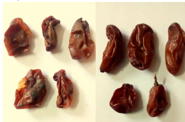
Fig. 10 Comparison of grapes dried in open sun drying method and in the solar tunnel greenhouse dryer without the biomass heater
