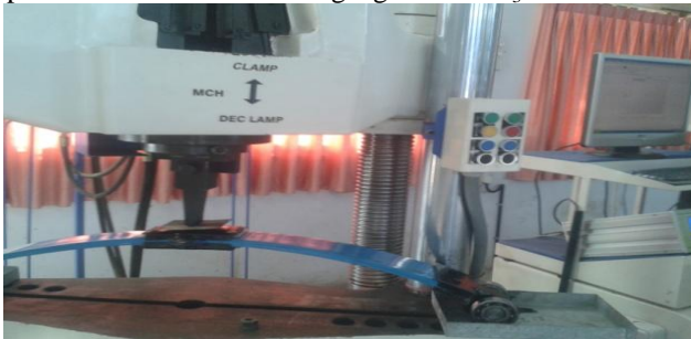
Fig. 7 Testing of C-Glass/epoxy composite leaf spring.
