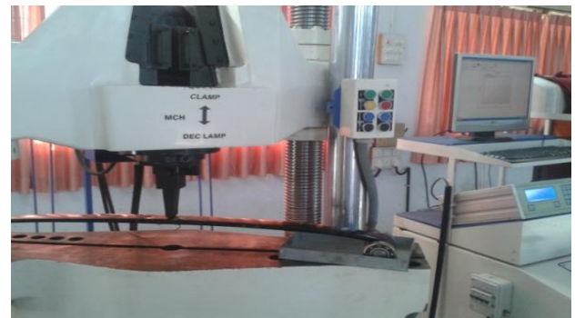
Fig. 6 Testing of steel leaf spring.
