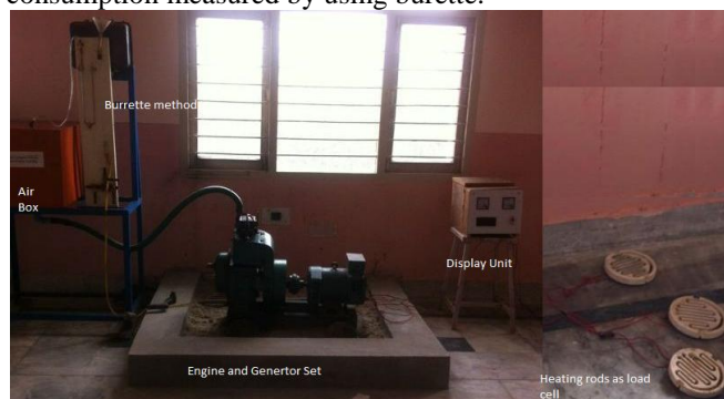
Fig. 1 Test Rig with all Equipment
