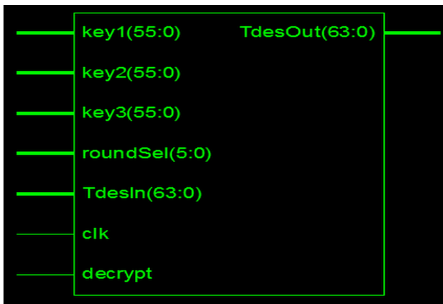
Fig.12 RTL schematic of TDES
