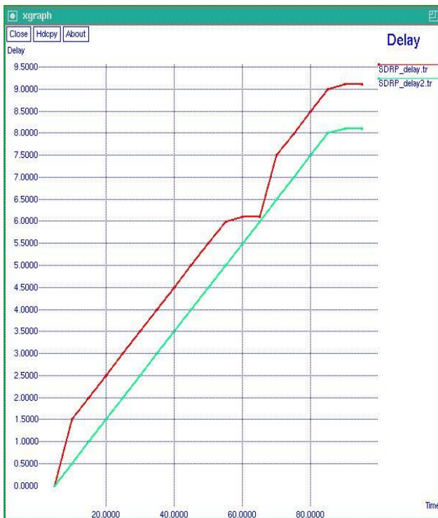
Figure 7. Packet Delay of SDRP and PDF-SDRP
