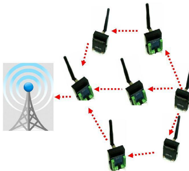
Figure 1. Example of a Wireless Sensor Network
