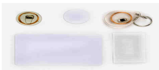
Fig.2. Different Types of MIFARE Classic Cards Source: [18]
