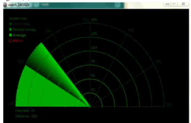
Figure (7): display for one static target at a distance of 150cm.
