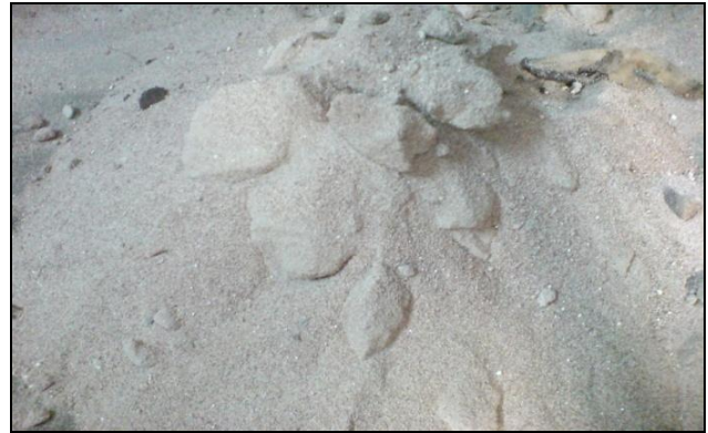
Fig. 2 Collapsed Structures Of Specimens Fired at 1100°C
