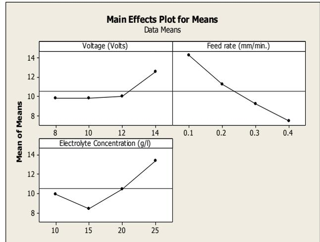
**Fig.3. Main Effect Plot for Means (Surface Roughness)**
