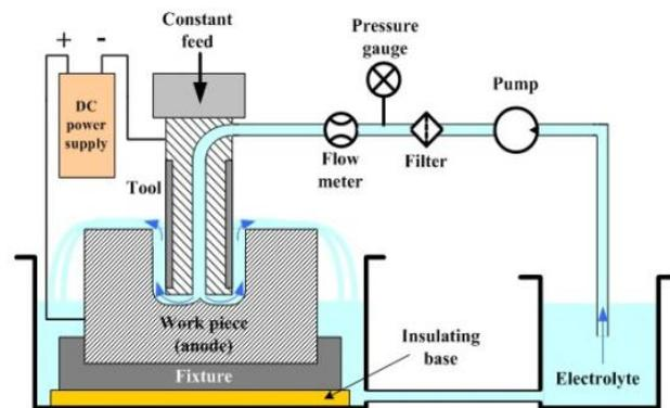
Fig.1. Schematic View of ECM
