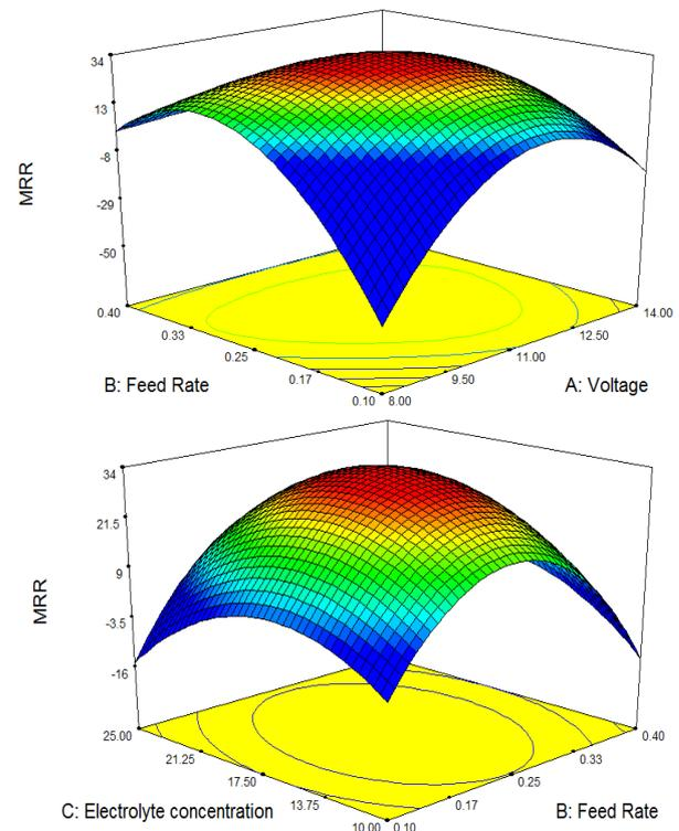
Fig.8. Influence on MRR in relation to change of (i) voltage and feed rate and (ii) Feed rate and electrolyte concentration
