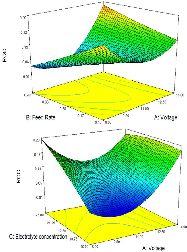
Fig.6. Influence on ROC in Relation to Change of (i) Voltage and Feed Rate and (ii) Voltage and Electrolyte Concentration
