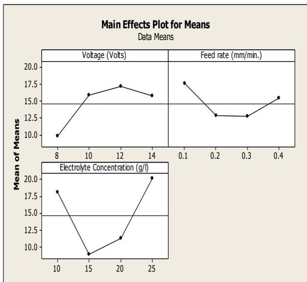
Fig.7. Main Effect Plot for Means (MRR)
