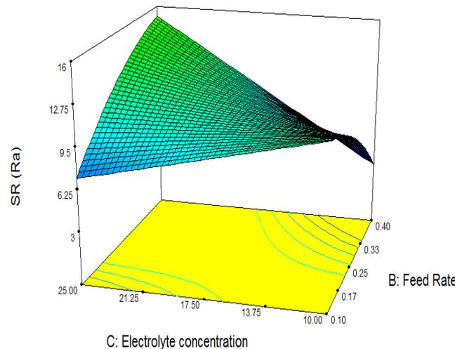
**Fig.4. Influence on Surface Roughness in Relation to Change of (i) Voltage and Feed Rate, (ii) Voltage and Electrolyte Concentration and (iii) Feed rate and Electrolyte Concentration**
