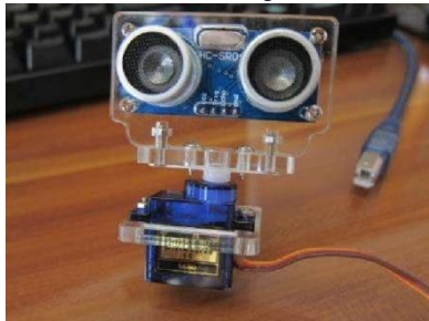
fig 13: servo motor with ultrasonic sensor
