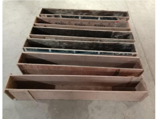
Figure 1 Flexural Beam moulds
