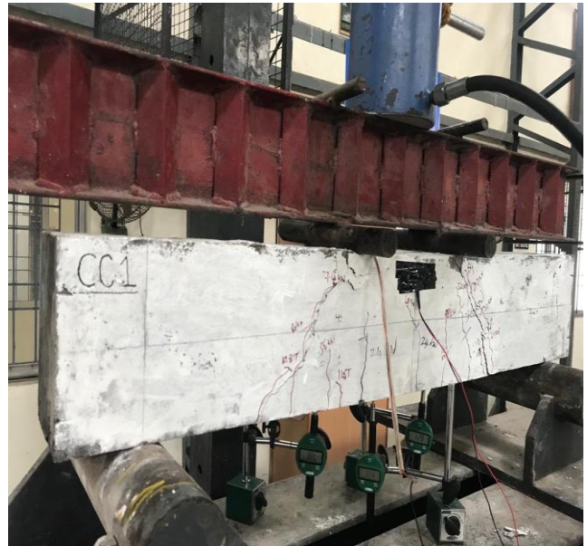
Figure 5 RCC Flexural Beam Testing Arrangements
