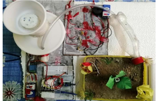
Figure 4: The circuit of the proposed IoT based auto-irrigation system
