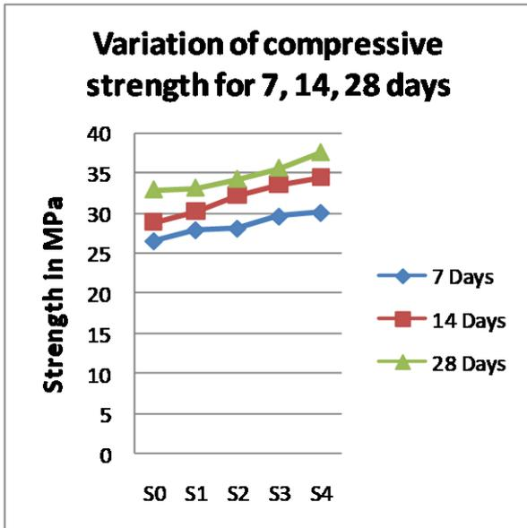
b) **Rebound Hammer Test.** Rebound Hammer test is carried on the cubes to check the compressive strength with the help of Rebound hammer. Rebound hammer test is done on hardened surface becomes most popular worldwide for in-situ concrete non-destructive testing. Testing is done for 7 Days, 14 Days and 28 Days
