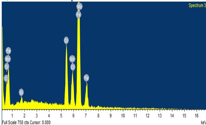
**Figure 7: EDAX of 316L SS Electrochemical Corrosion Test**
