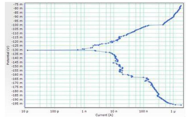
Figure: 4: 316L SS + Ringer Solution
